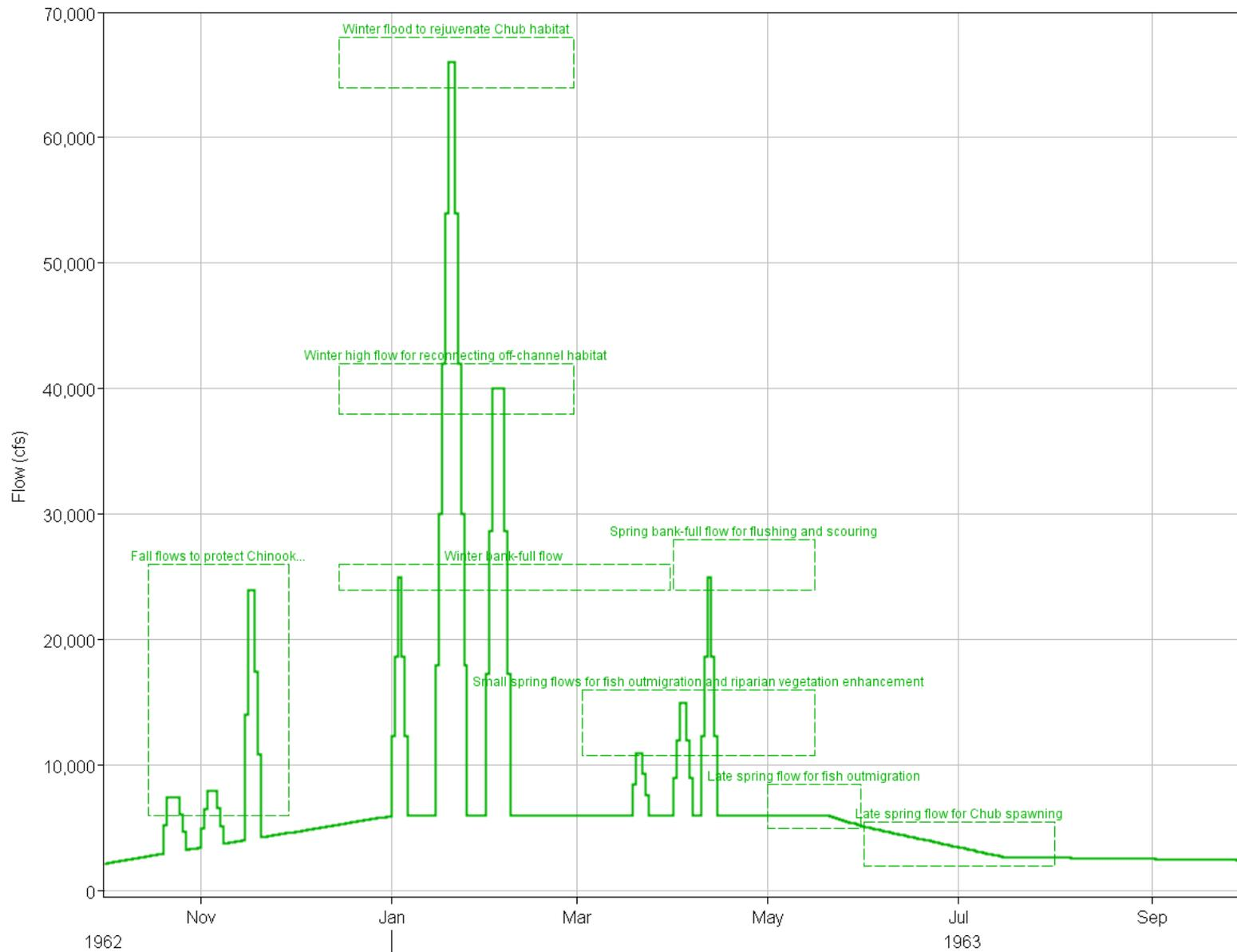
Figure 8. RPT generated plot of flow recommendations for the lower McKenzie River (Reaches 11-12)
