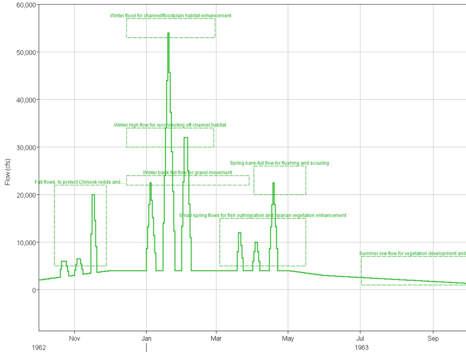
Figure 6. RPT generated plot of flow recommendations for the EWEB canal reaches (Reaches 8–10)
