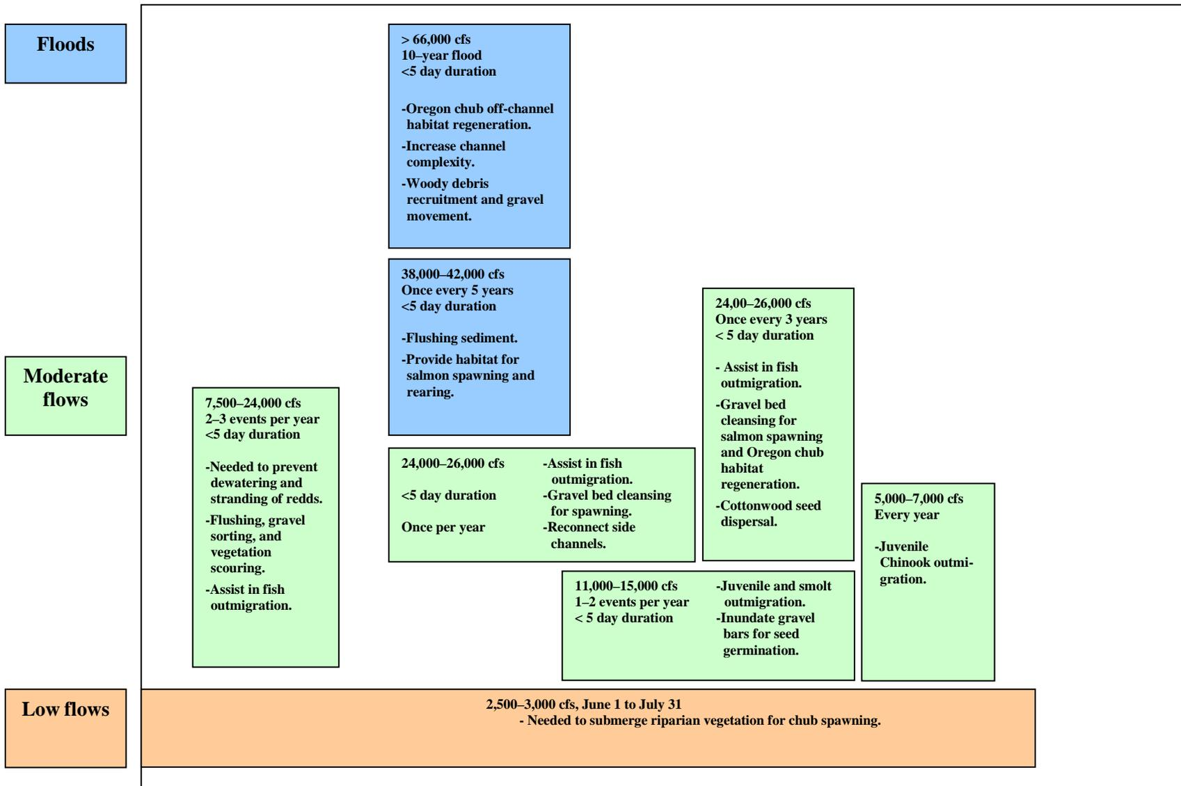
Figure 9. Dam flow release and ecology linkages for the Lower McKenzie River (Reaches 11–12)
