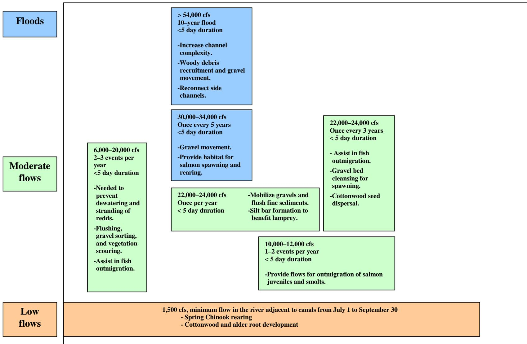
Figure 7. Dam flow release and ecology linkages for the EWEB canal reaches (Reaches 8–10)
