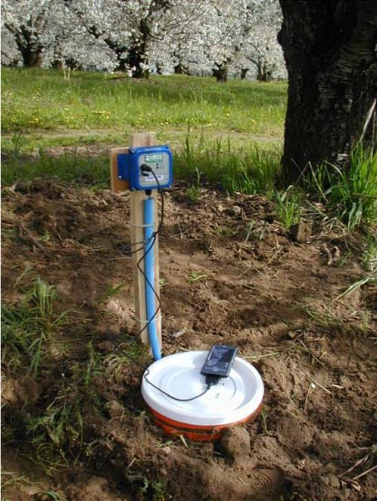
Logger with below grade meter installation.
